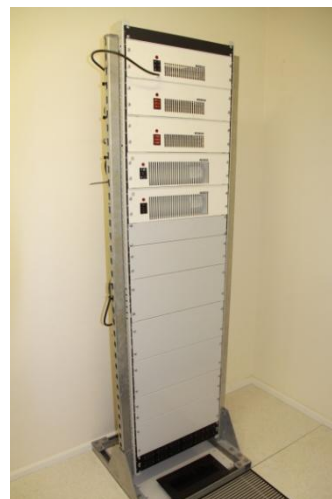
MKI & MKII 3U 2kW Heat Loads mounted in test frame
